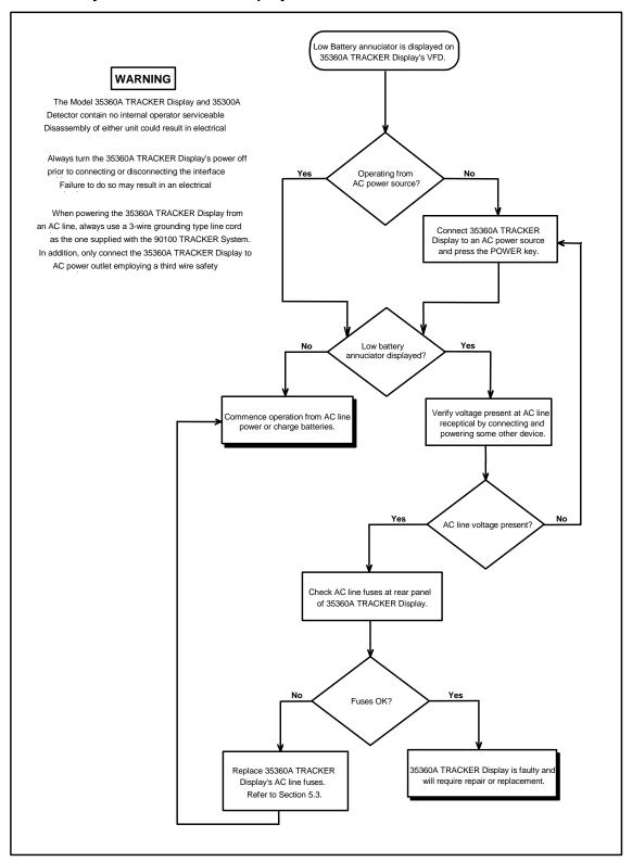
Figure 4-2 Low Battery Flowchart
